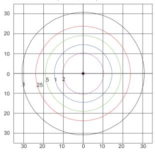
Isofootcandle Plot shows light distribution pattern at ground level with LED chip with no shield. Readings have been taken assuming the photometric center of the luminaire to be 11.13 feet above ground level. IES files for standard lamps are available on our website.
