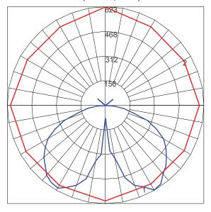
$\label{eq:maximum Candela = 623.46; Located at Horizontal Angle = 90; Vertical Angle = 30 \\ \#1 - Vertical Plane Through Horizontal Angles (90 - 270) (Through Max. Cd.) \\ \#2 - Horizontal Cone Through Vertical Angle (30) (Through Max Cd.) \\ \\$
