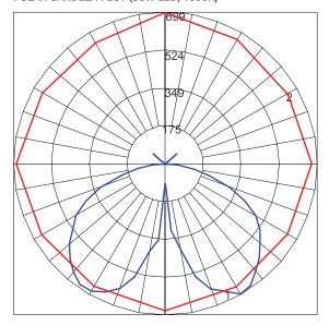
Maximum Candela = 698.91; Located at Horizontal Angle = 90; Vertical Angle = 30 #1 - Vertical Plane Through Horizontal Angles (90 - 270) (Through Max. Cd.) #2 - Horizontal Cone Through Vertical Angle (30) (Through Max Cd.)
